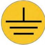
All electrically conductive parts found in the workplace of 5 meters around each booth opening, and particularly the objects to be coated, have to be grounded. The grounding resistance of each object must amount to maximally 1 MOhm. This resistance must be checked/tested regularly when starting work.
